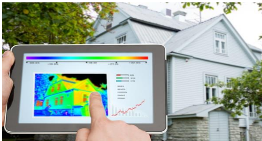
Figure 2: A thermographic representation to detect air leaks and insulation gaps
