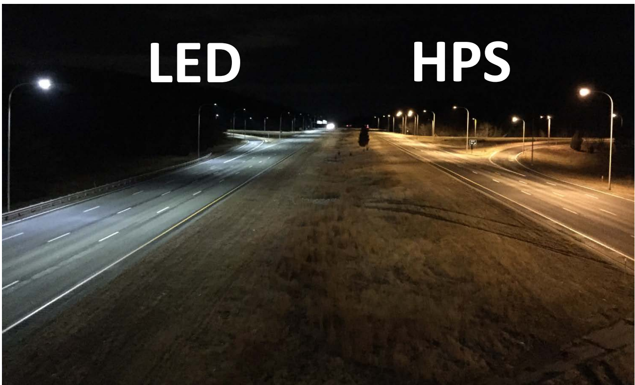
Dec 2015 @ I-295 (Exit 7): LED versus High Pressure Sodium (HPS).
