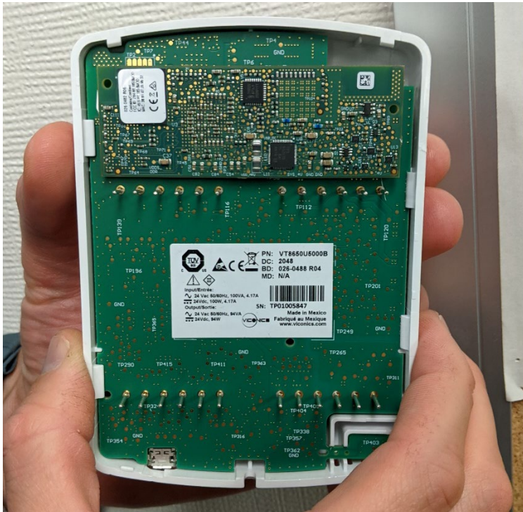
Figure 1-4. Zone 1 thermostat with Wi-Fi card exposed
